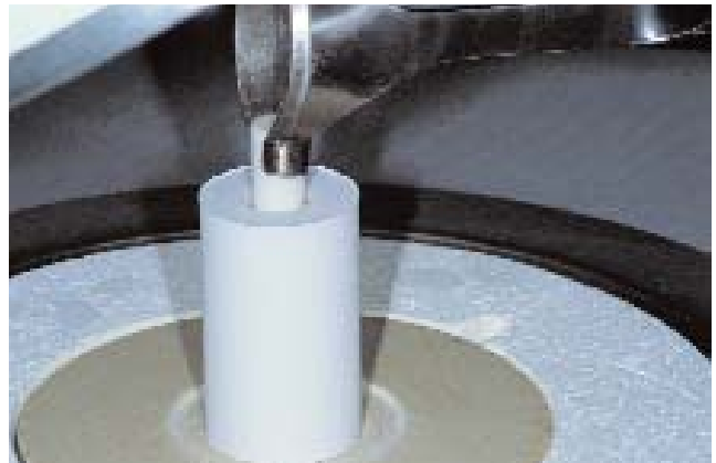
Insertion of the pre-heated AlOx plunger in the investment ring
