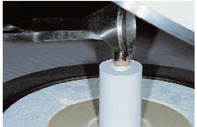
Insertion of the cold ingot in the investment ring
