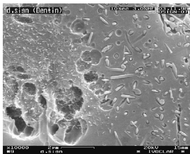
Fig 2: 10,000x magnification (SEM) of fluorapatite crystals in the IPS d.SIGN Dentin material after etching of the preparation. The distinct etching pattern indicates the simultaneous presence of leucite crystals.
