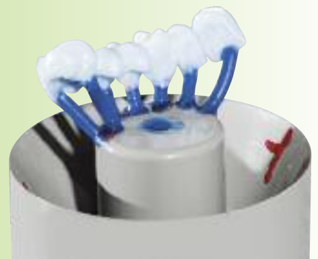
The cylinder-shaped sprue former facilitates the process
