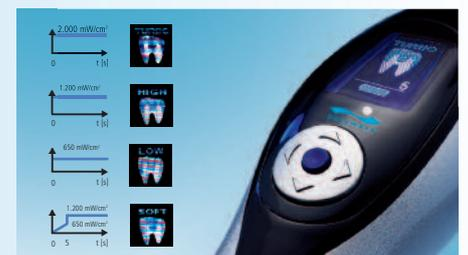
The four easy-to-use programs: Turbo for maximum performance, High Power for fast curing, Low Power for curing in areas near the pulp and Soft Start for stress-reduced polymerization.
