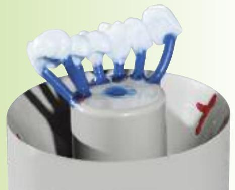
The cylinder-shaped sprue former facilitates the process
