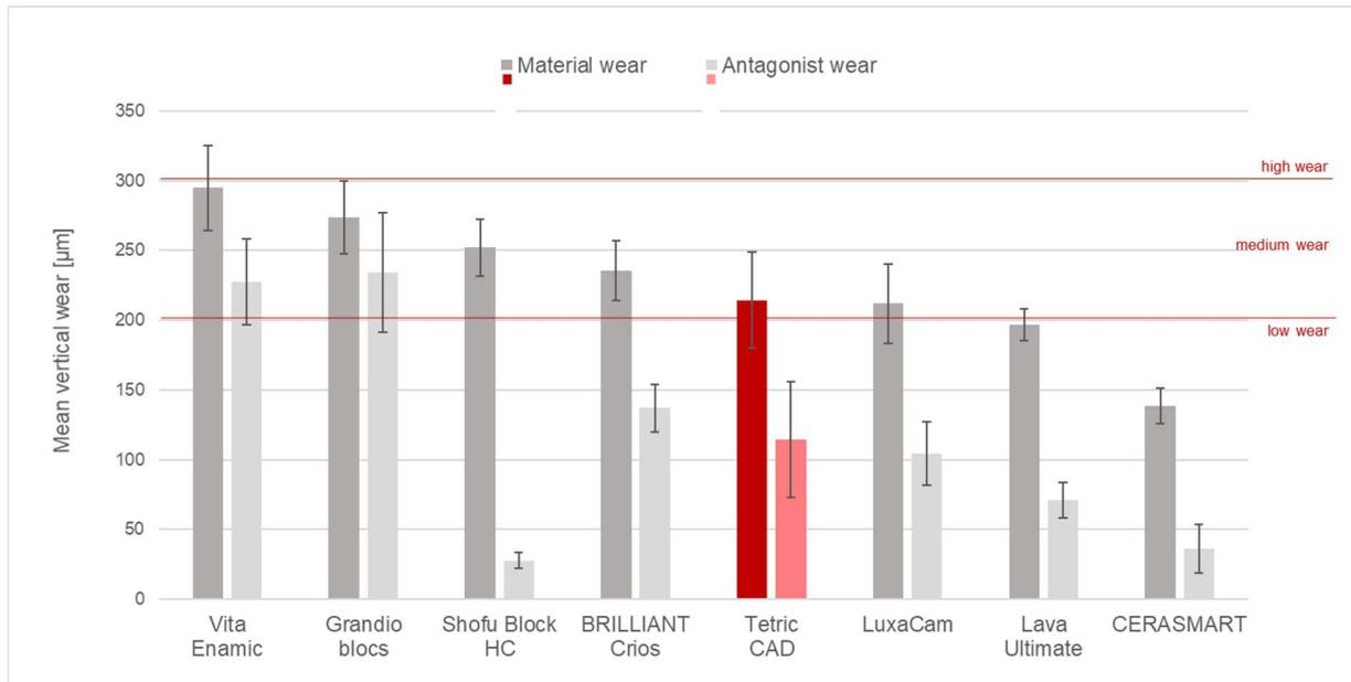
Fig. 10: Comparison of wear resistance (Willytec Method) of various composite block materials. R&D Ivoclar Vivadent. Schaan, March 2018
