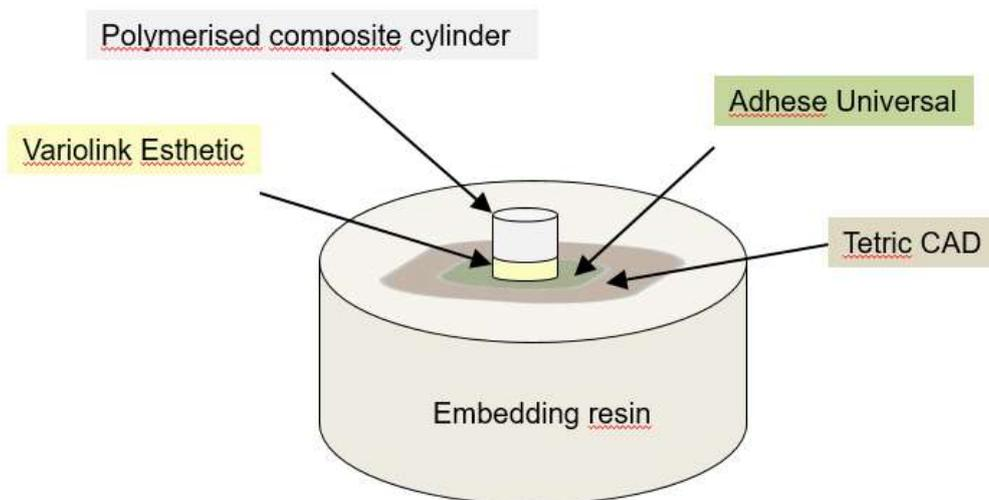
Fig. 11: Schematic representation of method for shear bond strength testing for indirect restorations
