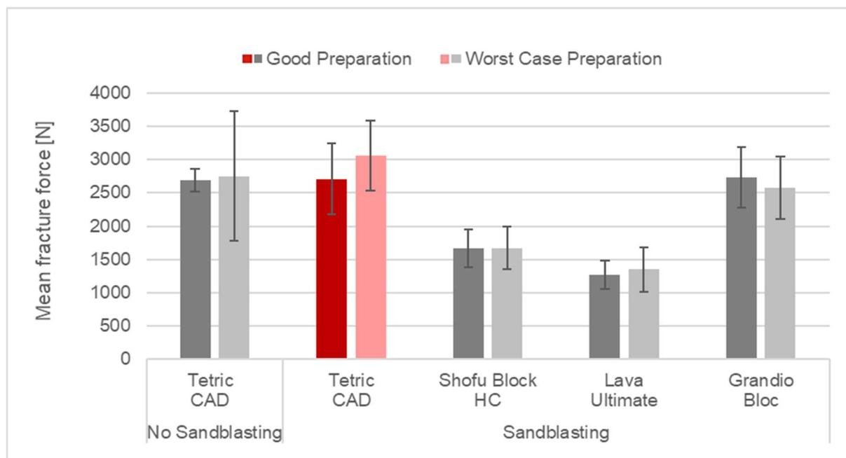
Fig. 14: Mean fracture force after water storage and thermocycling/mechanical loading for various CAD/CAM composite materials. Rosentritt 2017 (16)
