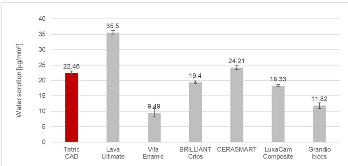
Fig. 8: Comparison of water sorption with Tetric CAD and various composite CAD/CAM block materials. R&D Ivoclar Vivadent Schaan. April 2018
