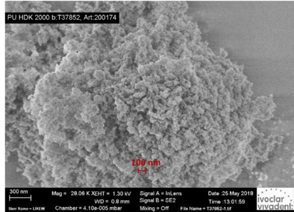
Fig. 4: SEM image of silicon dioxide microfillers with mean particle size of < 20 nm
