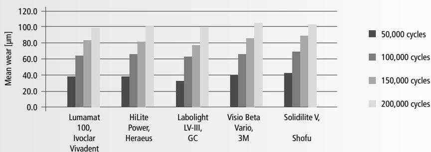
Wear resistance of SR Nexco according to the ACTA method in approved polymerization units.
