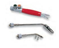
Single-orifice torches produce a pointed, hot flame of up to 2900 °C/5252 °F in temperature. A propane-oxygen mixture enables spot soldering without excessively heating up the surrounding areas
