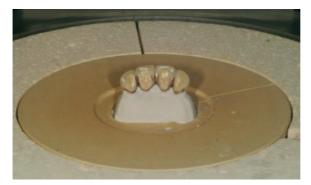
The processing temperature of the solder must be reached. The temperature may be a maximum of 50 °C/122 °F higher than the processing temperature to allow the solder to flow into the soldering gap. However, the processing temperature of the solder must be at least 50 °C/122 °F below the last firing temperature of the ceramic material.
