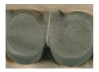
During the soldering procedure a reciprocal diffusion between the liquid solder and the solid-hot alloy takes place.
