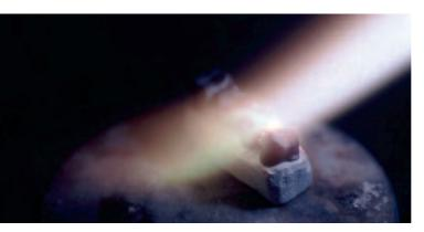
Once the working temperature of the object to be soldered has been reached as a result of the heat from the flame being applied to the exposed soldering contact surfaces, the solder quickly and reliably flows into the soldering gap and fills it.
