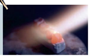
A solder with the correct processing temperature is selected according to the alloys to be soldered. Dental solders must be corrosion resistant and demonstrate a composition similar to that of the alloys to be joined.
