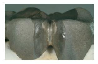
Allow the solder joint to cool slowly. Remove the soldering investment. Blast the object with 50 or 100 micron Al<sub>2</sub>O<sub>3</sub> to remove oxides and flux residue. Instead of blasting precious metal alloys can be pickled (PCT AScid).
