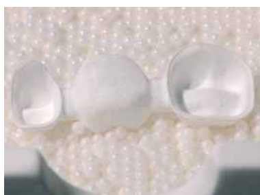
Fig 12: 3-unit bridge framework on IPS e.max ZirCAD on ZrO 2 beads after the sintering process
