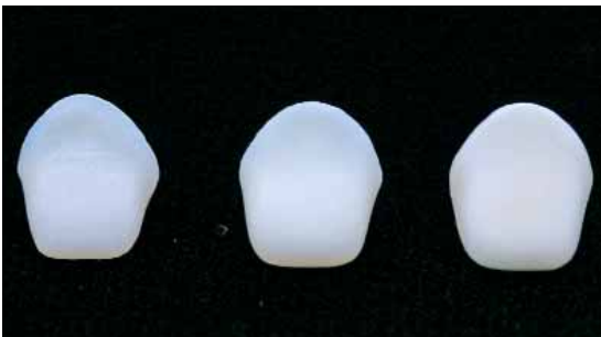
Fig 1: Unveneered frameworks: IPS e.max CAD, IPS e.max Press and IPS e.max ZirCAD
