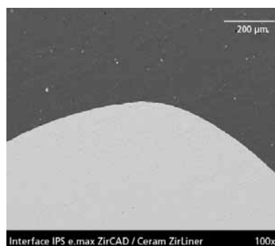
Fig 13, 14: Bonding region between IPS e.max Ceram, ZirLiner and IPS e.max ZirCAD (100x and 1000x magnification, polished section, BDE Contrast)
