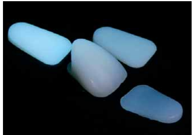
Fig 9: IPS e.max Ceram crown with the respective shade tabs under UV light; Shoulder, Dentin and Enamel materials to show the course of fluorescence
