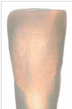
Fig 7: Test sample of an opal component by transmitted light
