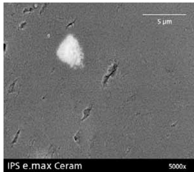
Fig 2: Conventional opaquing with SnO 2 as the opaquing agent; SEM image, 5000x magnification
