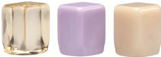
Fig. 5: Glass block, blue partially-crystallised block (lithium metasilicate) and crystallised block (lithium disilicate)
