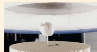
Conduct the Stains and Glaze firing on a honey-combed tray using the stipulated parameters.
