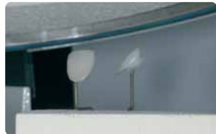
Place the objects on the honey-comb firing tray and start the firing program.
