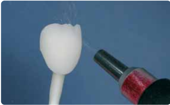
Carefully blast the restoration with \text{Al}_2\text{O}_3 at 0.5 bar pressure (Caution: abrasive)
