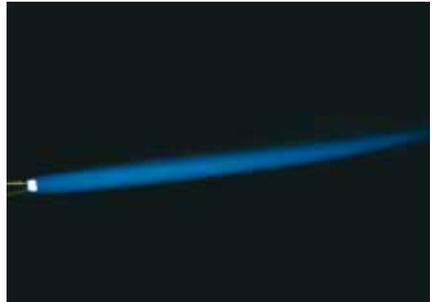
Multi-orifice torches produce a large, soft flame. In conjunction with a propane-compressed air mixture or a propane-oxygen mixture, these torches are suitable for even heating of the object to be soldered.
