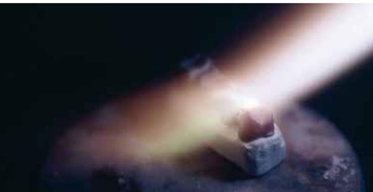
Once the working temperature of the object to be soldered has been reached as a result of the heat from the flame being applied to the exposed soldering contact surfaces, the solder quickly and reliably flows into the soldering gap and fills it.
