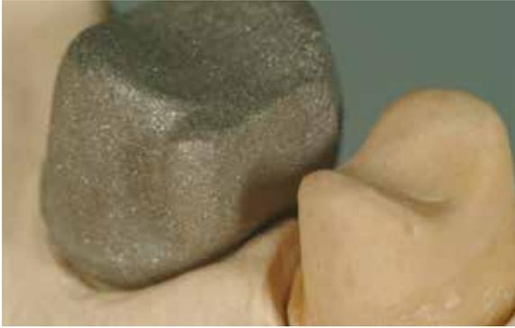
Clean soldering contact surfaces are a basic requirement for optimum wetting. The surfaces of the soldering contact areas have to be prepared by grinding and/or sand blasting.
