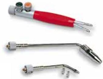
Single-orifice torches produce a pointed, hot flame of up to 2900 °C/5252 °F in temperature. A propane-oxygen mixture enables spot soldering without excessively heating up the surrounding areas.
