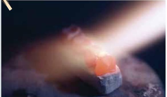
A solder with the correct processing temperature is selected according to the alloys to be soldered. Dental solders must be corrosion resistant and demonstrate a composition similar to that of the alloys to be joined.
