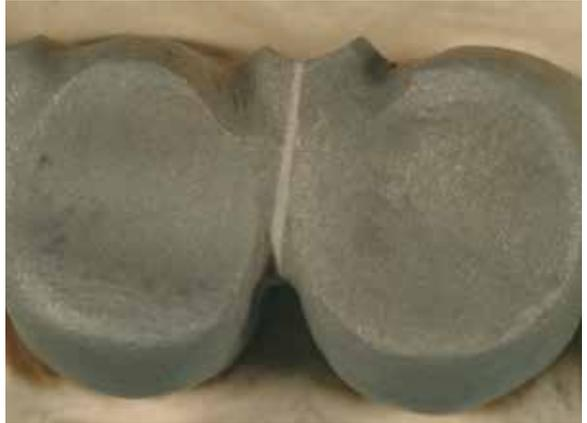
During the soldering procedure a reciprocal diffusion between the liquid solder and the solid-hot alloy takes place.
