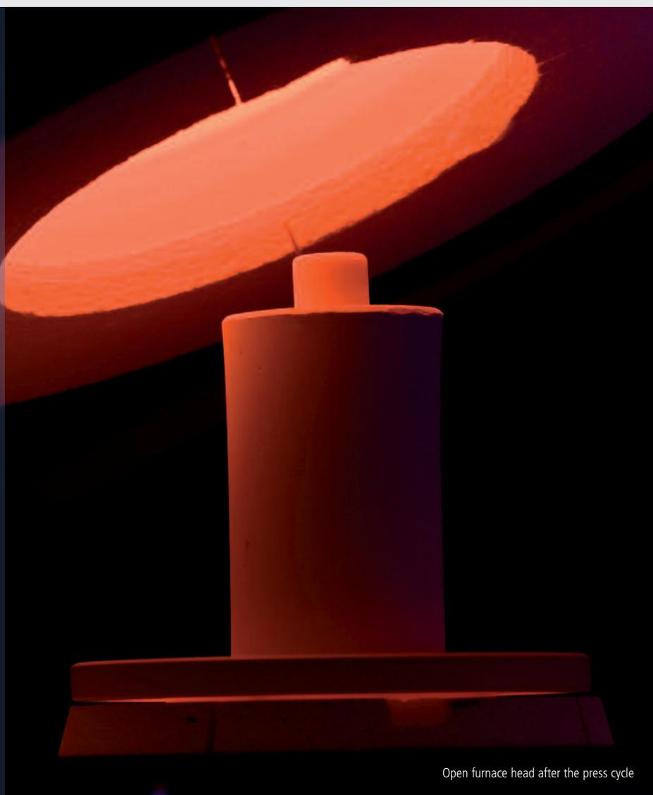
Open furnace head after the press cycle
