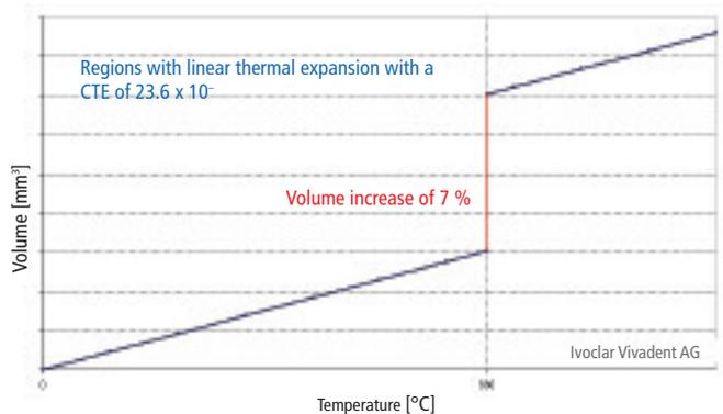
Fig 1: Thermal expansion of aluminum as a function of temperature
