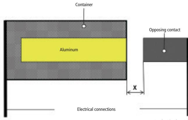
Fig 2: Open aluminum contact
