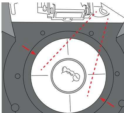
Fig. 21: The objects are positioned with the largest surface area facing the infrared camera.
