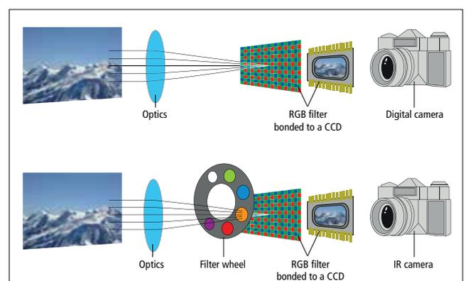
Fig. 7: The technical principle of the digital camera and the IR camera
