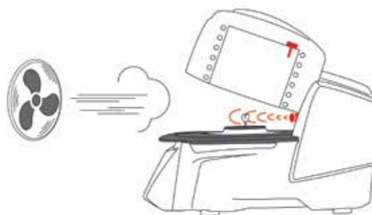
Fig. 20: Infrared technology measures the temperature directly on the surface of the object. Therefore, any possible draughts do not affect the measuring results.
