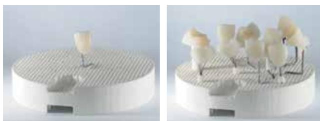
Fig. 15: Two examples showing different ways of loading the firing chamber
