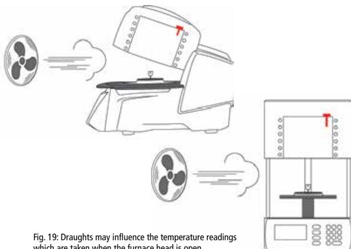
Fig. 19: Draughts may influence the temperature readings which are taken when the furnace head is open.
