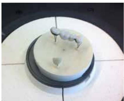
Fig. 22: Large objects must be positioned in the front, facing the IR directly.
