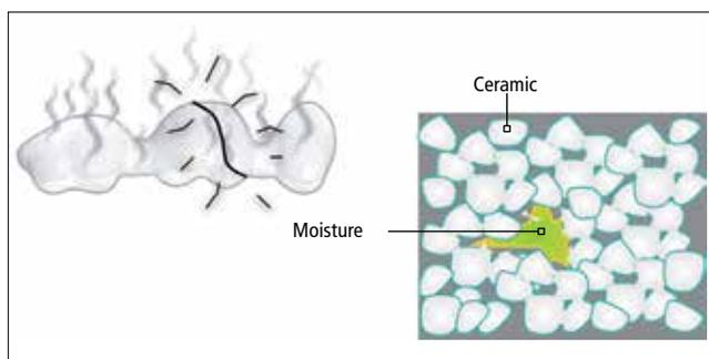
Fig. 14: Risk of fractures if the moisture in the ceramic evaporates too quickly
