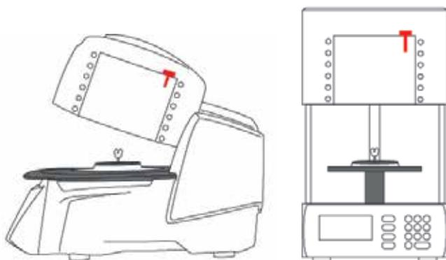
Fig. 18: Different types of furnaces with swivelling furnace heads or a lifting mechanism
