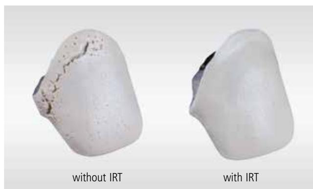
Fig. 17: Opaquer fired with and without infrared technology
