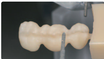
Telio CAD restoration after milling in the CAD/CAM unit and being detached from the holder
