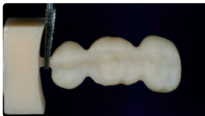
Telio CAD restoration after milling in the CAD/CAM unit and being detached from the holder
