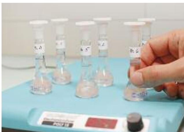
Figure 5: Extraction of the methyl methacrylate by stirring in acetone for 72 hours
