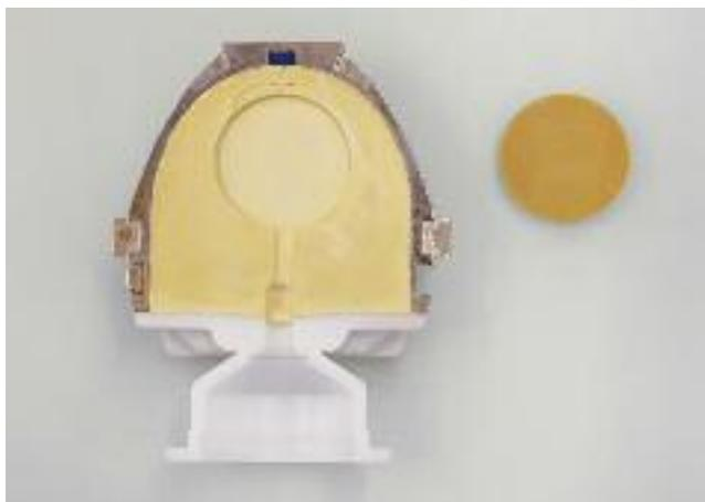
Figure 2: Investment of the silicone moulds to determine the residual monomer content.
