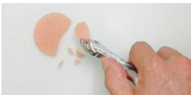
Figure 4: Crushing the test specimen to determine the initial weight
