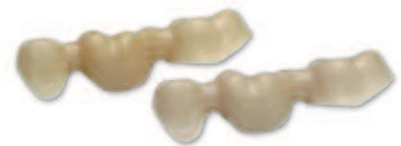
above: Shaded with liquids from another manufacturer below: Shaded with IPS e.max ZirCAD Colouring Liquids
