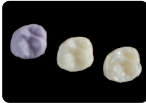
IPS e.max CAD molar crown: milled – crystallized – glazed
